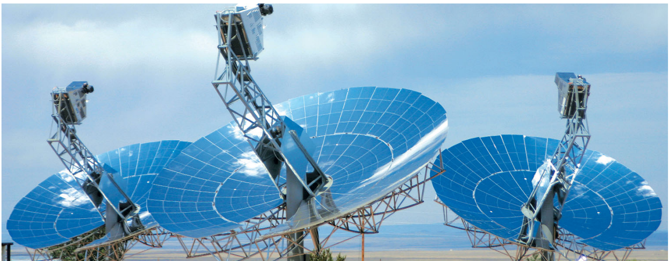
Solar dishes with sterling engines are a technology of major potential for low-density locations, suitable for public spaces within suburbia. Credit: Tessera Solar.
