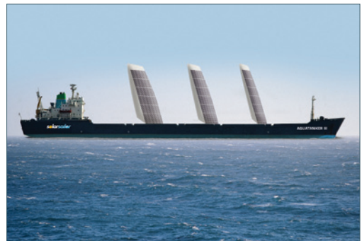
Image and patented 'solarsails' courtesy of Solar Sailor www.solarsailor.com.au . New approaches to reducing energy use and emissions in shipping include the use of kites, sails (some integrating PV), and blowing bubbles under the hull.
