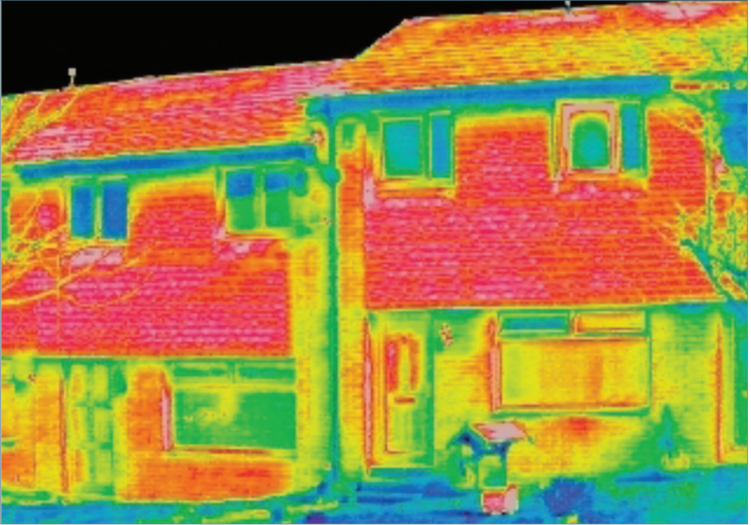
Credit: Jonathan Pope, CP Energy Ltd. Infrared photography is a very effective tool for discovering the energy leakage of our houses. Retrofitting with high-efficiency insulation materials and energy management systems has huge implications for their energy performance.
